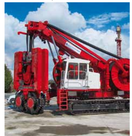
HC05, the new small Hydrofraise machine.
